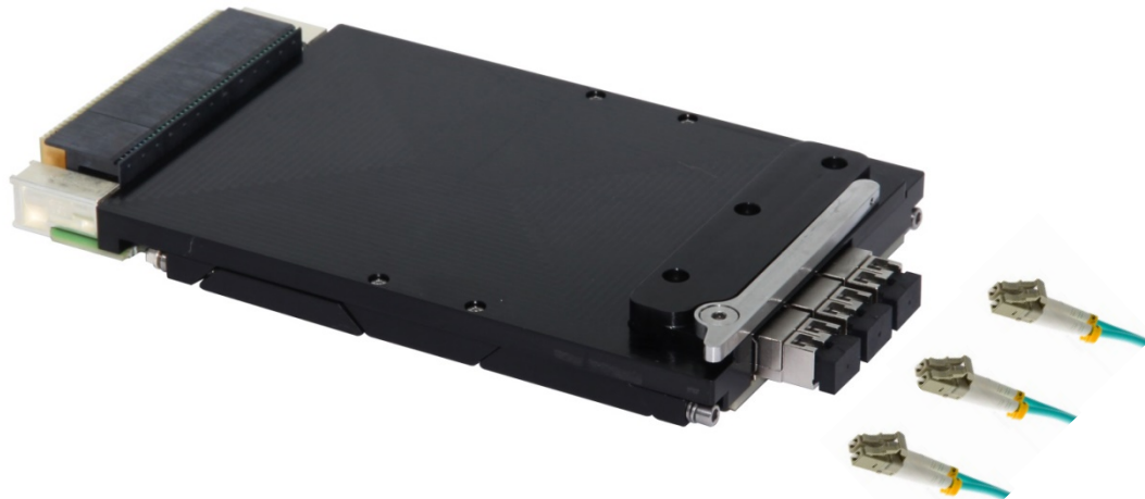
Interface Concept ComEth4590a switch w/ 3 front panel 10G optical connectors
