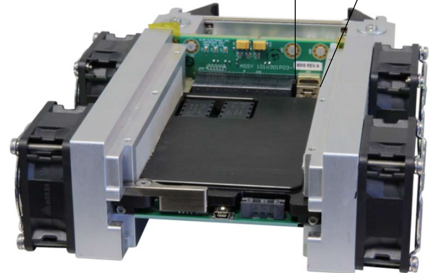
Interface Concept ComEth4082e switch implementing VITA 66.5:
